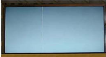
Vertical Line Source TAB IC Defect
