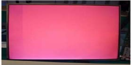
Vertical Block Source TAB IC Defect
