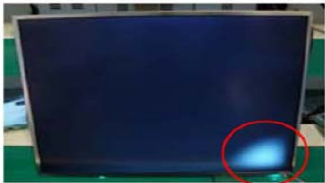
Panel Mura, Light leakage
